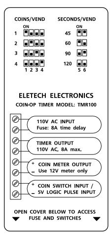
The TMR100 is a digital timer with coin accumulation function. It is designed for use in coin operated kiddie rides and other similar equipment. In addition to the AC output for the motor (and the sound box if any), there is also a DC output for mechanical coin meter (pulse counter) for revenue tracking.
